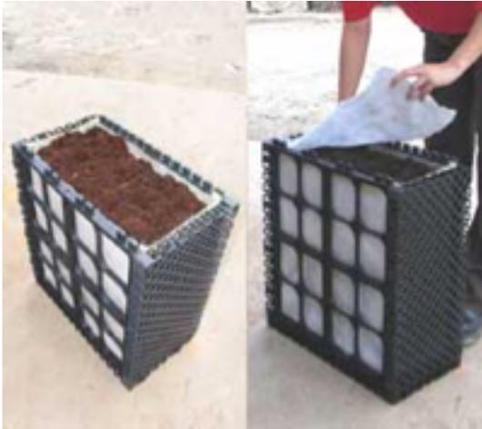
Assemble the VGM Module bottom, sides, front and back. Place the VGM Module top aside. Set the soil retention bag in place and fill. A highly inorganic lightweight soil mix (>95% inorganics, 30-50 lbs per cu. ft) should be used in the module. Then snap the VGM Module Top into place.
