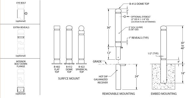
B-4 bollards shown above in 5" pipe, also available in 8" diameter. Bollards are available in 30", 36", 42" and 48" lengths.
