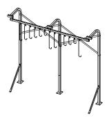
Insert the Track Rack or Bike File assembly into the Channel Supports and secure. See Track Rack or Bike File instructions for more detail. 4b
