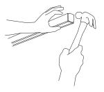
Insert a ½" Carriage Bolt into the last slot and fasten 3 Washers and a Tamperproof Nut. Finish by hammering in an End Cap.
